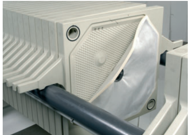
Chamber plate Clean System and cloth with integrated rim seal (patented)
