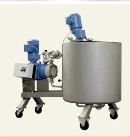
The dosing device DOS 500 for kieselguhr and other filtering aids ensures uniform mixing and precisely adjustable dosing of the filtering aid. Foam formation can be (optionally) avoided thanks to a frequency-controlled mixing device. Kieselguhr filtration is used to filter wine, for example, inside a chamber filter press, or beer in plate and frame filters.
